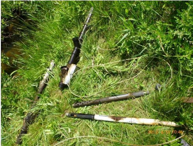
Figure 1: Multi-parameter sondes and installation equipment
