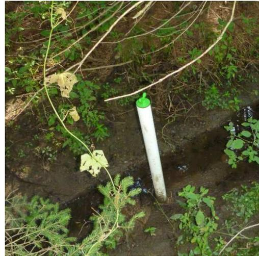
Figure 2: Level logger stand pipe installation in stream
