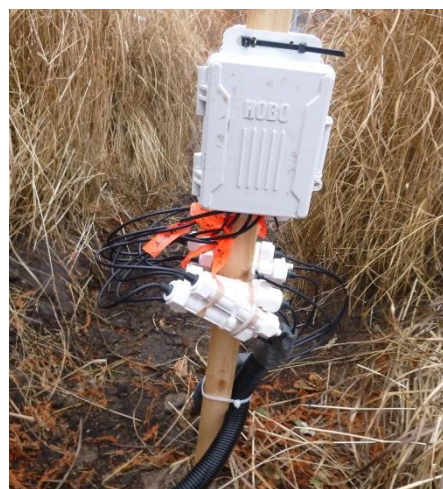
Figure 13: Soil moisture data logger installed in a swale
