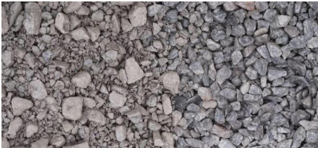
Figure 6: Granular "O" (left) and \frac{3}{4} inch clear stone (right) base material
