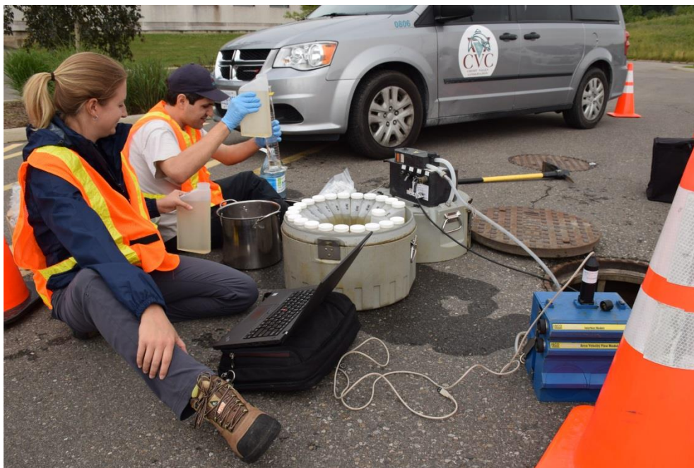
Figure 11: Staff collecting a composite water quality sample
