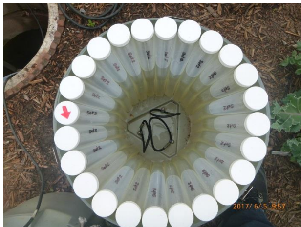
Figure 10: Autosampler base with 24 1-litre bottle configuration
