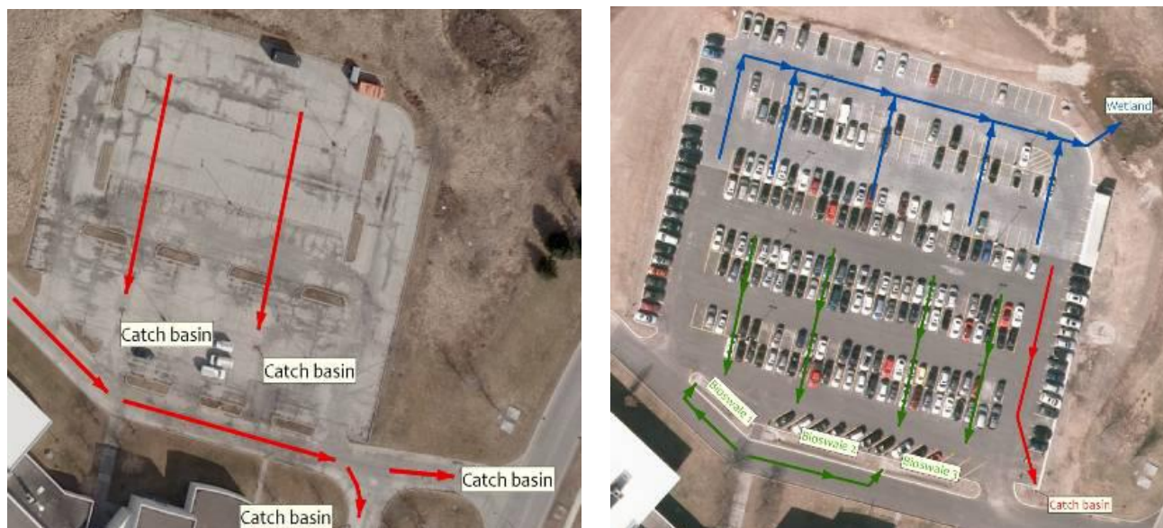
Figure 2: IMAX parking lot traditional asphalt drainage pre-retrofit (left) and LID treatment post-retrofit with permeable pavement indicated in blue and asphalt to bioretention indicated in green (right)
