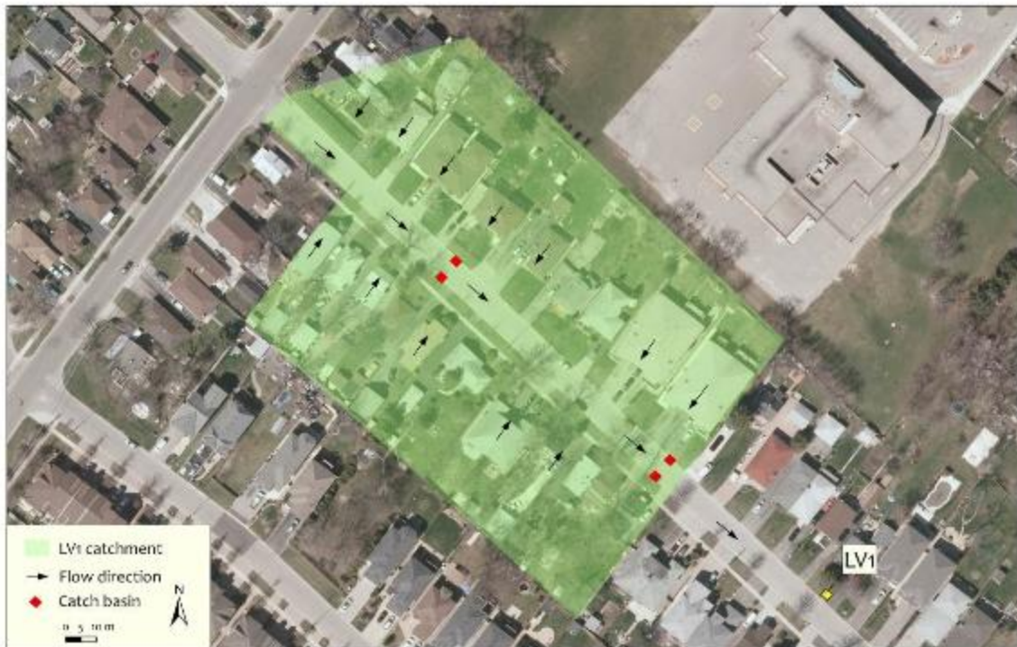
Figure 3-9 LV-1 Water quality reference site drainage area with direction of runoff
