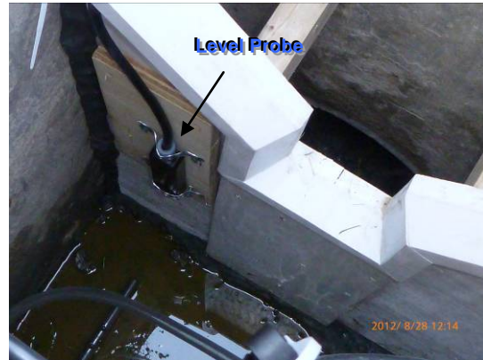
Figure 2-2: Level Probe Fastened to Weir Face
