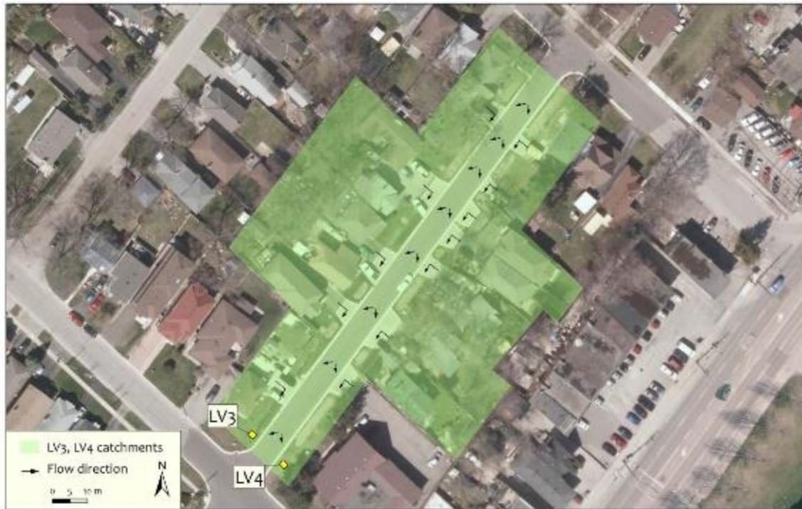
Figure 3-11 LV-3 LID retrofit collecting runoff flows from center to north side of street and LV-4 LID retrofit collecting runoff from center to south side of street.
