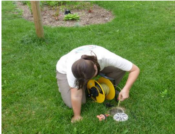
Figure 2-6: Manual level measurements to verify accuracy of readings and to calibrate level logger as needed
