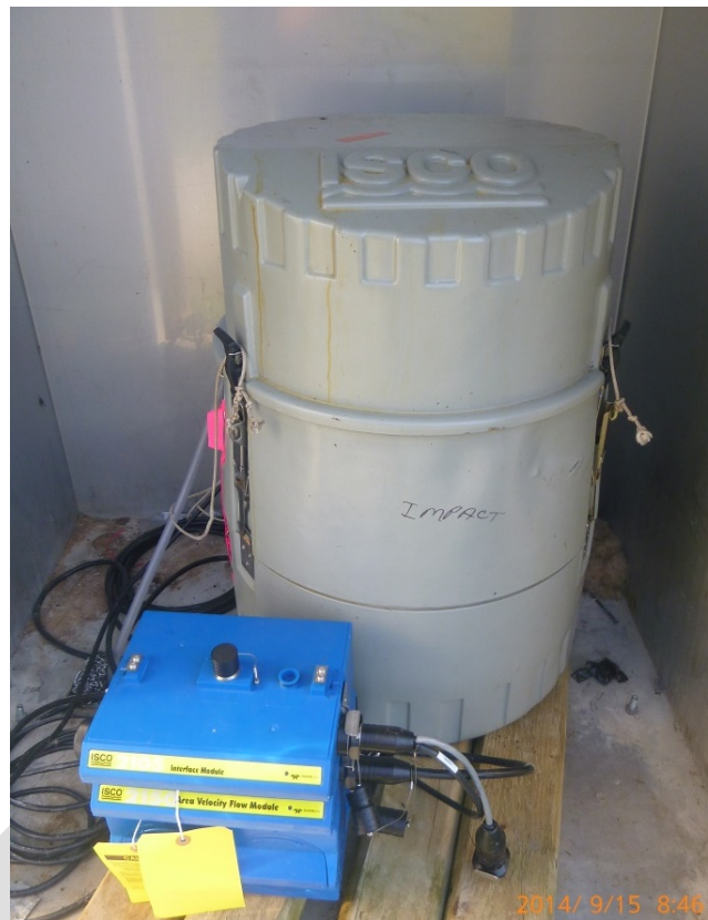
Figure 3: Example of the monitoring equipment that is used in the catchbasin
