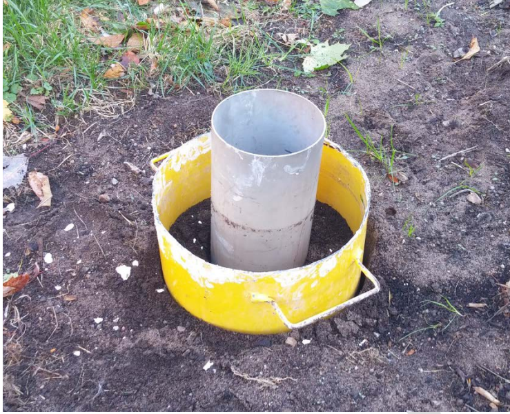
Figure 5: Double ring infiltrometer used to measure infiltration rate in a bioswale
