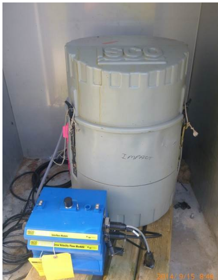
Figure 4: Monitoring setup showing the ISCO Area-Velocity Flow Module and an Auto Sampler
