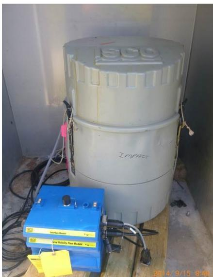
**Figure 2: Monitoring setup showing the ISCO Area-Velocity Flow Module and an autosampler**
