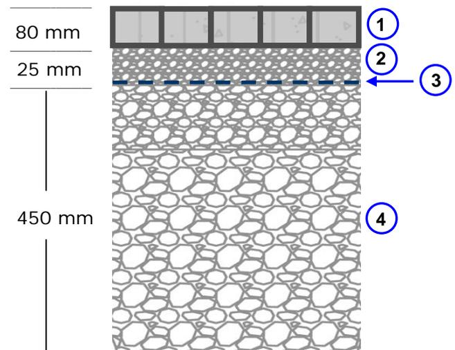
Section view of the permeable pavement, illustrating the various
