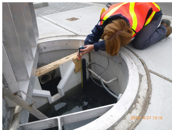
Figure 15: Monitoring staff conducting a water level measuring at the inlet monitoring chamber
