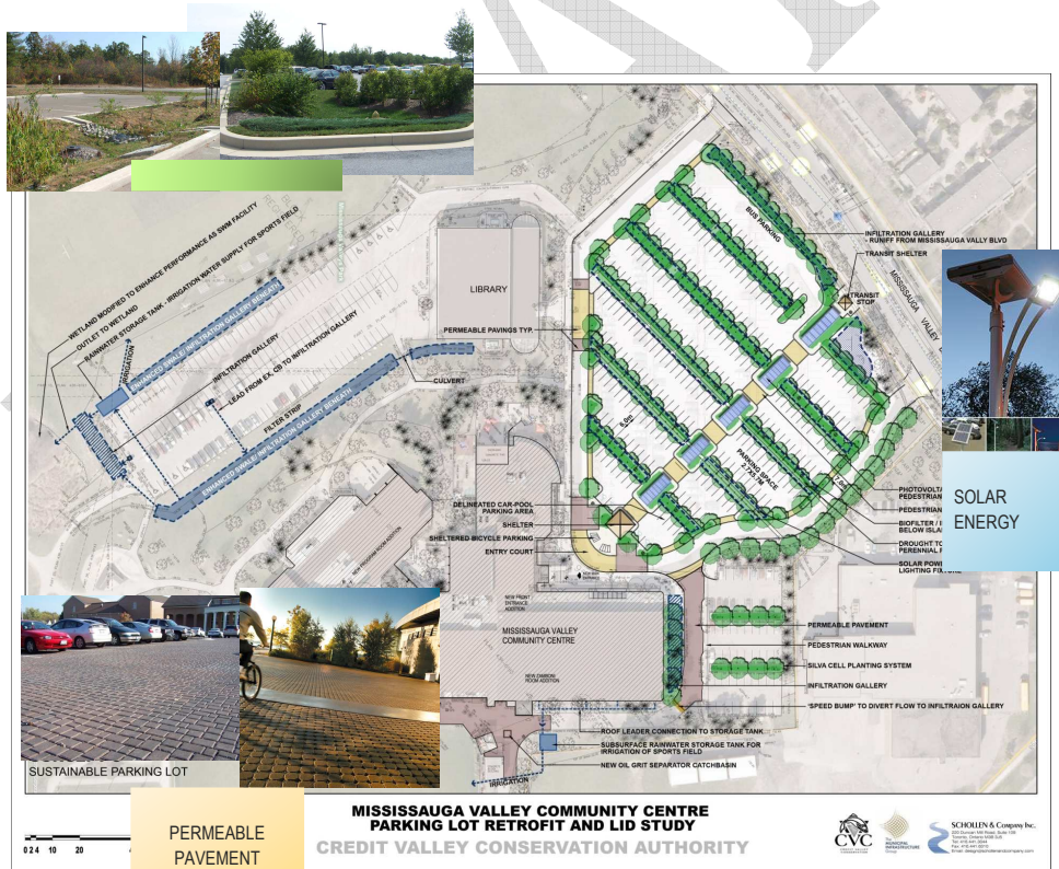
Figure 3.13 Total redesign of the main parking area to Provide water balance and water quality and quantity control
