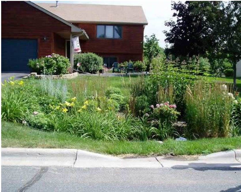
Figure 3.27 Example of a rain garden
