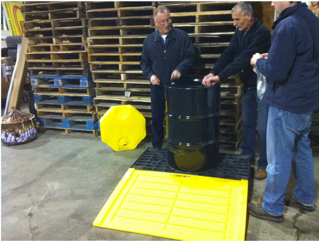
New spill containment pads installed
