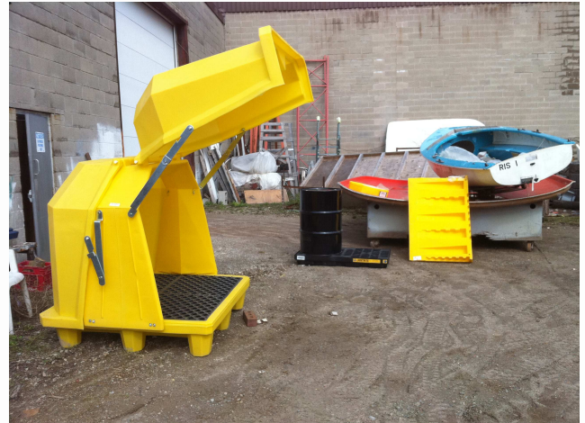
New covered spill pallet for 100 gallon drums
