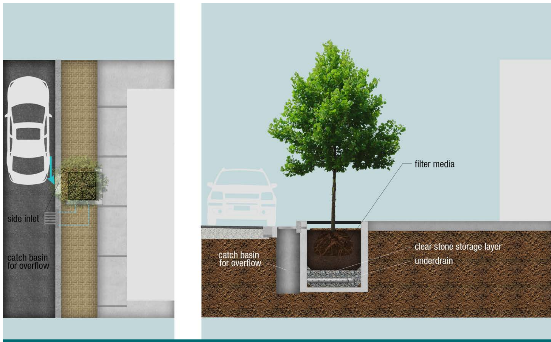
Figure 2.4.2: Pre-cast tree planter plan view [left] and cross-section [right]
