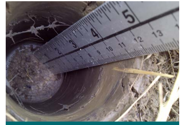
Figure 10.3.2: Coring has indicated that a layer of impermeable clay has clogged this bioretention unit. Major rehabilitation including replacement of the bioretention soil media will be required to allow for filtration and infiltration. (Source: Aquafor Beech)
