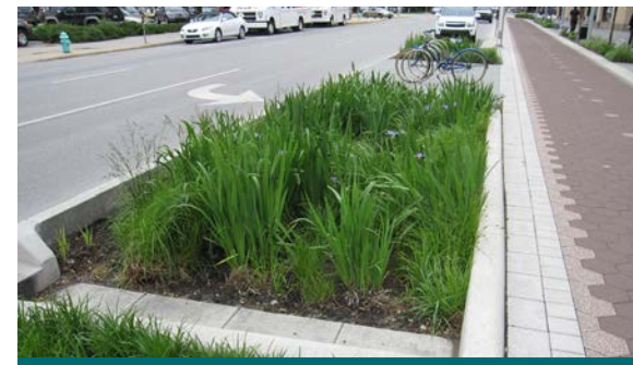
Figure 2.1.4: Bioretention curb extensions can be part of a street reduction, where a lane within the roadway can be dedicated to other uses such as street parking, bicycle lanes, pedestrian crossings, and street greening. (Source: CVC)
