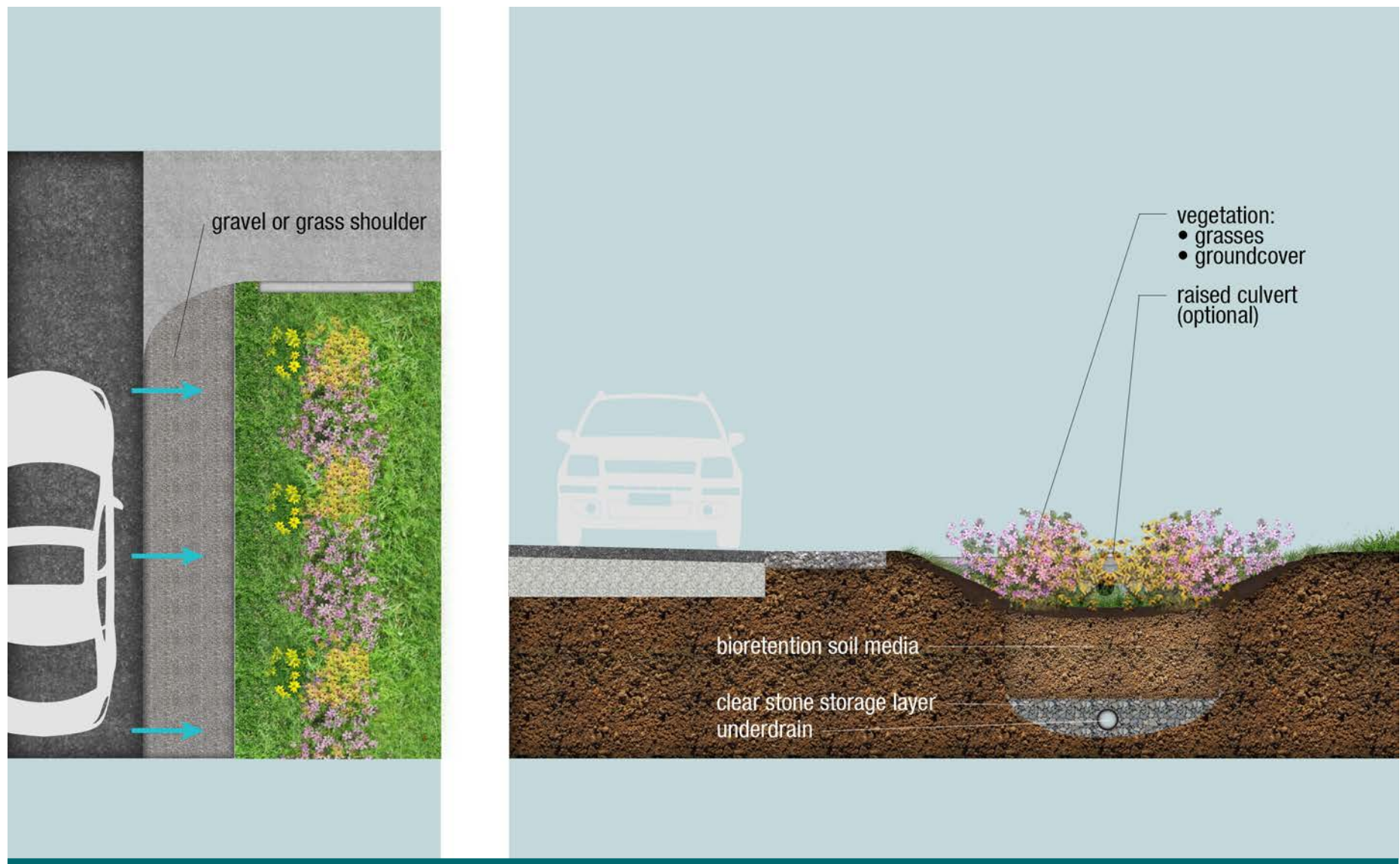
Figure 2.2.5: Bioswale plan view [left] and cross-section [right]
