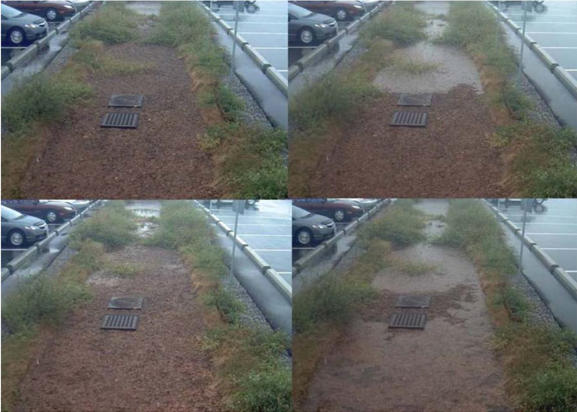
As part of the monitoring program a surveillance camera was installed to observe occasions where water ponding took place. This information was used to help determine when overflows through the surface catch basins occurred
