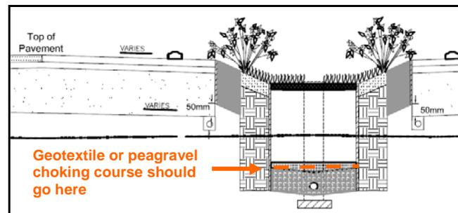
Cross section of bioretention cell, showing location where transition material should have been placed to prevent soil media from eroding through the sub-drain
