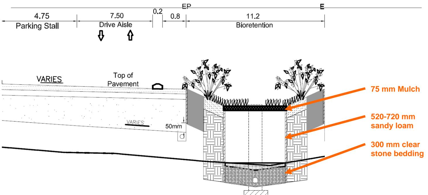
Cross section of one of the bioretention cells within the MTO carpool parking lot
