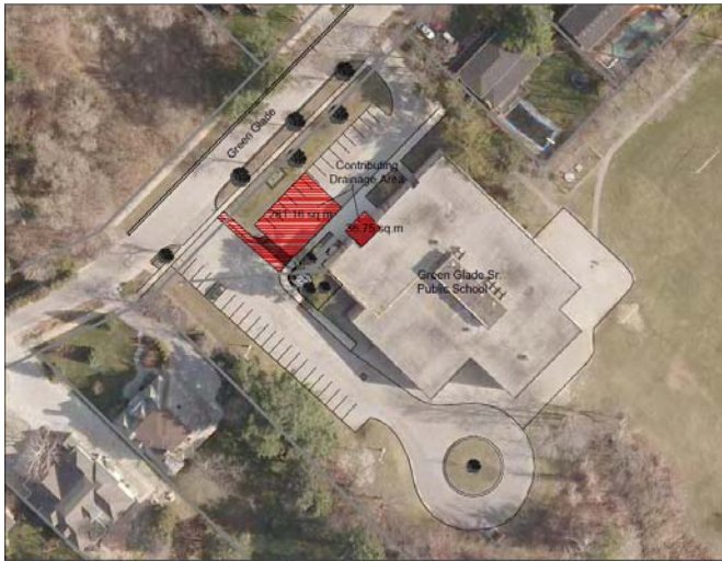
Contributing drainage area of rain garden
