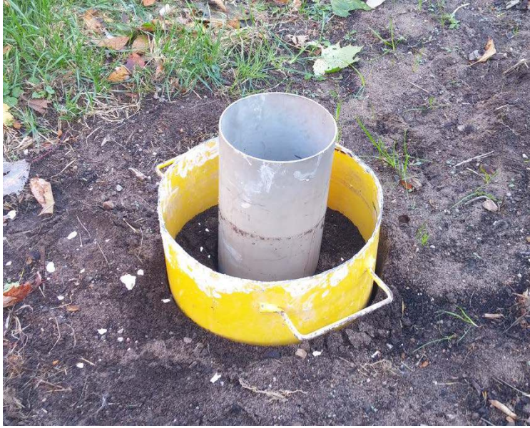
Figure 6-3 Double ring infiltrometer used to measure infiltration rate in a bioswale
