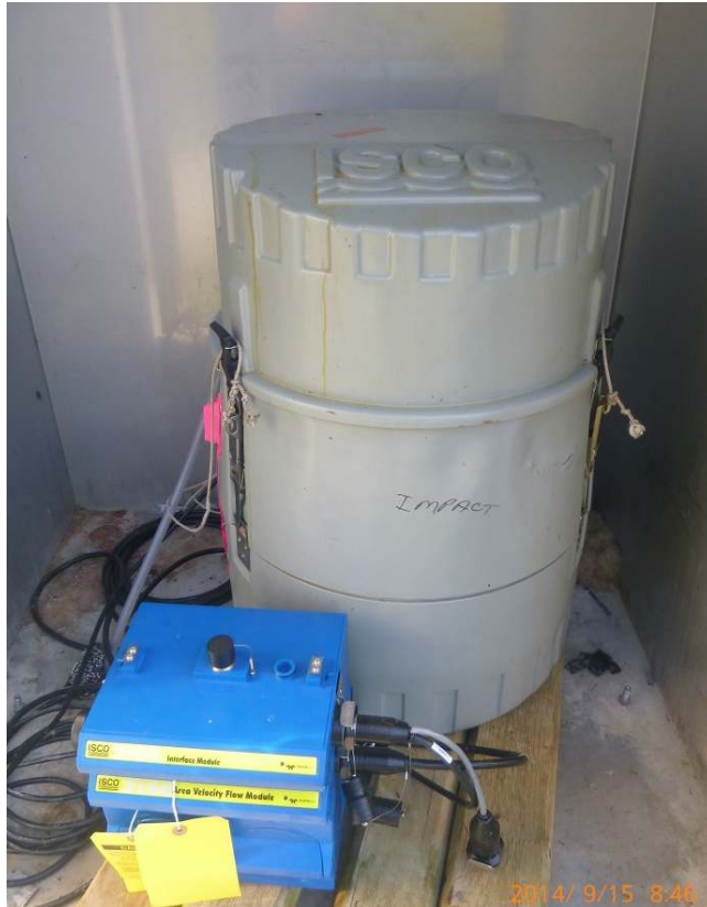
Figure 6-1 Example of the monitoring equipment that is used in the catchbasin
