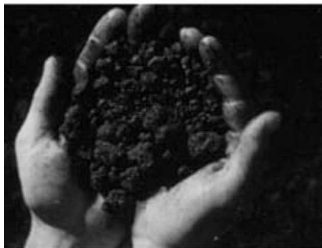
Figure 2. Oil sand is a mixture of bitumen, sand, water and clay.
