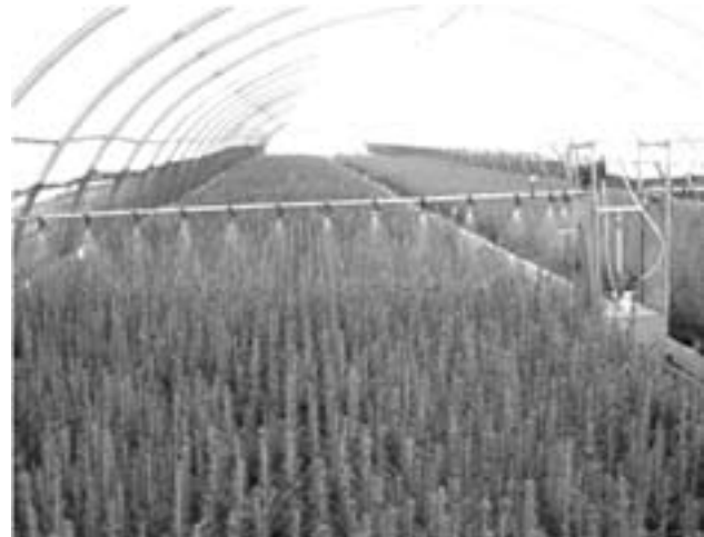
Figure 2. Irrigation of (2+0) white spruce seedlings under tunnel conditions by a Aquaboom motorized boom system.
