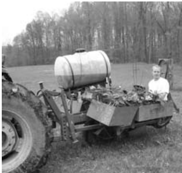
Figure 1. Tractor-hauled coulters with trencher and packing wheels, also equipped for herbicide application.
