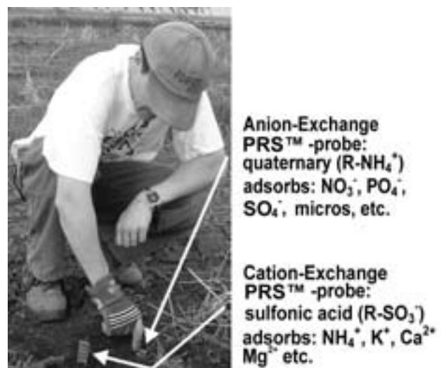
Figure 2. PRS™-probes used to measure soil nutrient availability in situ .
